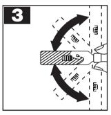
3. Close sample vial and invert a few times, until the freeze-dried contents are completely dissolved.
